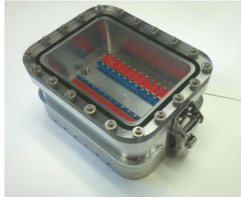
Tortuga's pneumatics manifold assembly
